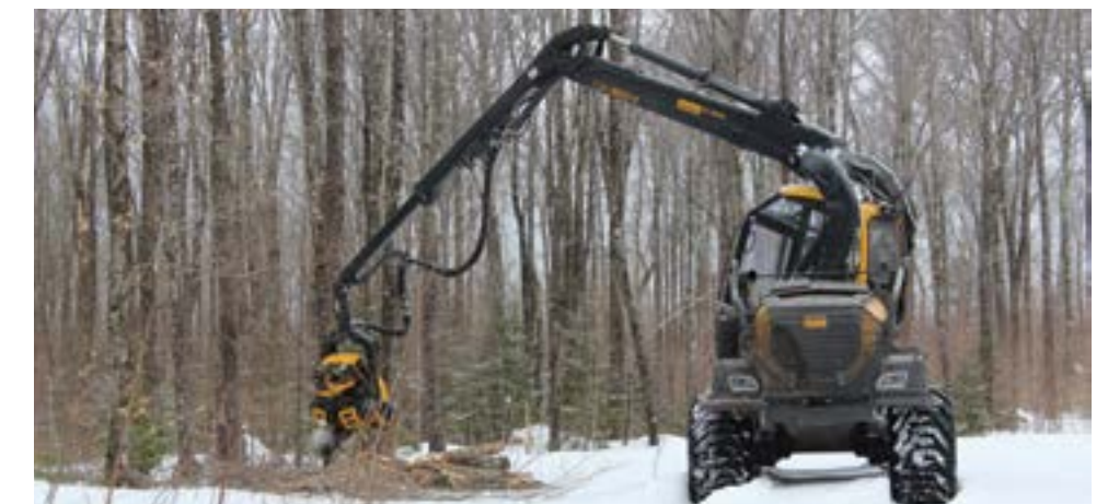
Ladwig's new Ponsse ScorpionKing Harvester is in its first season. He hopes it will allow him to harvest up to 250 cords of timber per week, approximately 2.1 tons, depending on the species of wood.
